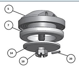
Place the seal retainer (item 5) in a vise holding on the flats. Utilizing a hammer and a punch remove the spring pin (item 20).
