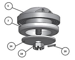
Check the sealing area (behind the seat seal (item 7)) of the seat retainer (item 5) for any excessive corrosion or pitting. If any are found, the seat retainer (item 5) should be replaced. Use care to ensure the sealing area is not scratched or damaged.
