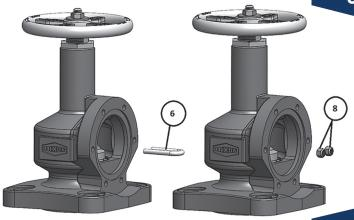
If necessary, use a wire brush to clean the threads of the u-bolt (item 6) and hex lock nuts (item 8) to remove any rust or scale. Inspect the threads for any excessive wear, corrosion, or pitting. If any are found, the components should be replaced.
