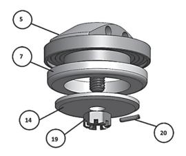
Install the soft seat (item 7) into the seat retainer (item 5). Place the disc washer (item 14) over the threaded portion of the seal retainer (item 5). Thread on the disc retainer castle nut (item 19).
