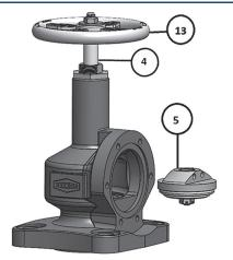
Using the handwheel (item 13), fully open the valve until the stem (item 4) runs out of upward travel.
