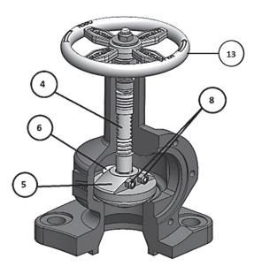
Using the handwheel (item 13), open the valve. Place the seal retainer (item 5) into the body with the holes at the top of the seal retainer facing the side outlet of the valve. Close the valve until the stem bottoms out on the seat retainer (item 5), then open the valve approximately 1/4 turn.
