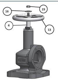
Install handwheel (item 13) onto the square portion of the stem (item 4). Place the handwheel washer (item 16) on top of the handwheel. Thread the lock nut (item 23) onto the end of the stem and with a 5/8" socket, firmly snug it against the handwheel washer.
